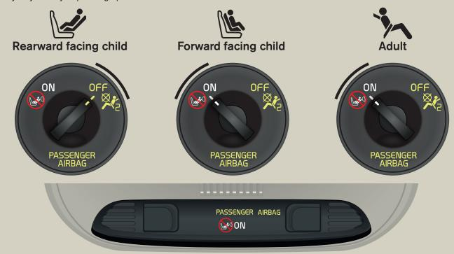
The ON/OFF position is clearly communicated in the Overhead Console (indication may vary in depending upon car model).
