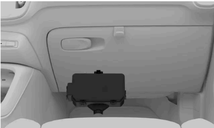
Fuse box location
