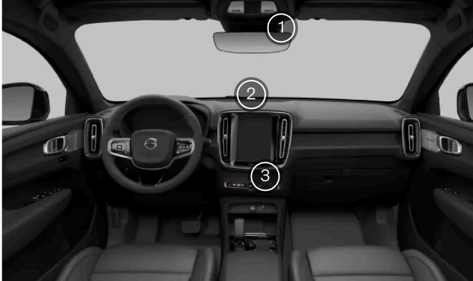
Interior climate sensors
