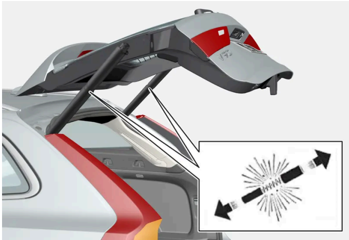
Preloaded springs for the power tailgate.
