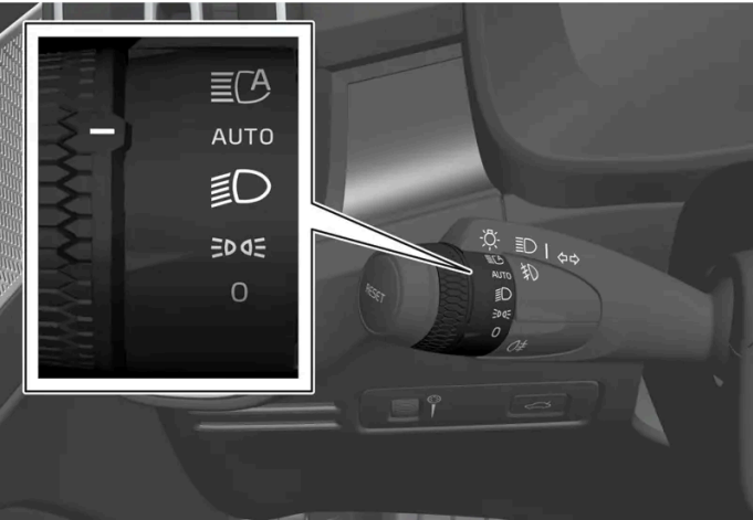
Lighting ring position.
