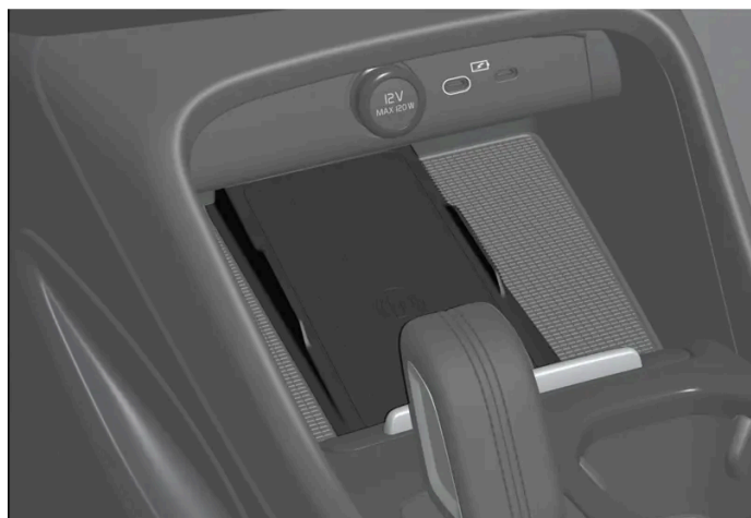
Wireless phone charger in front of gear selector
