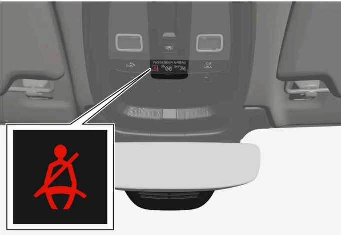
Reminder light in ceiling console.
