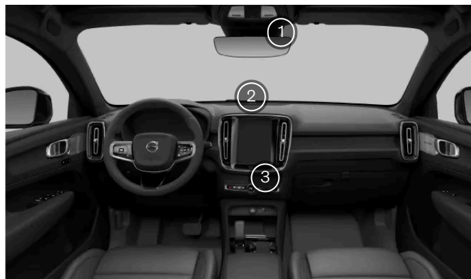
Interior climate sensors
