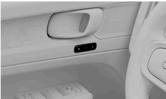
Location of the preset seat adjustment buttons
