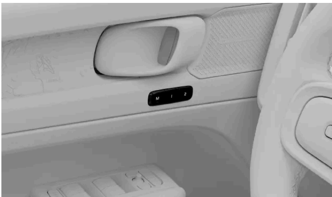
Location of the preset seat adjustment buttons
