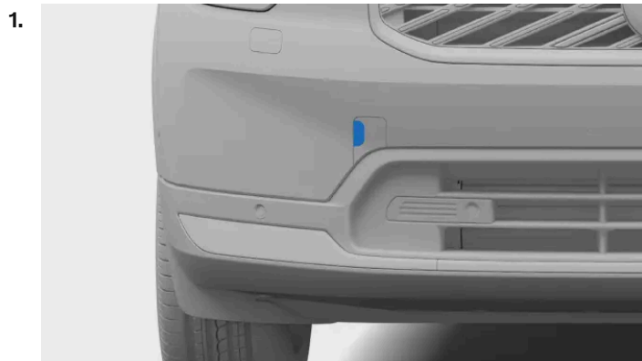
Front towing eye fastening cover
