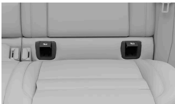
Locations of ISOFIX [1] anchor points for the outer rear seats
