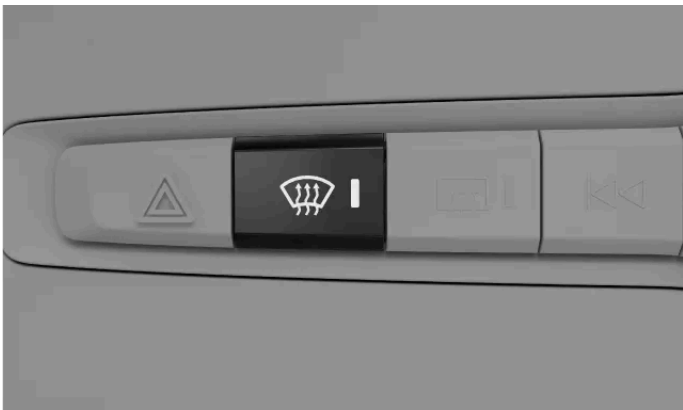
Max defroster button on the button panel below the center display
