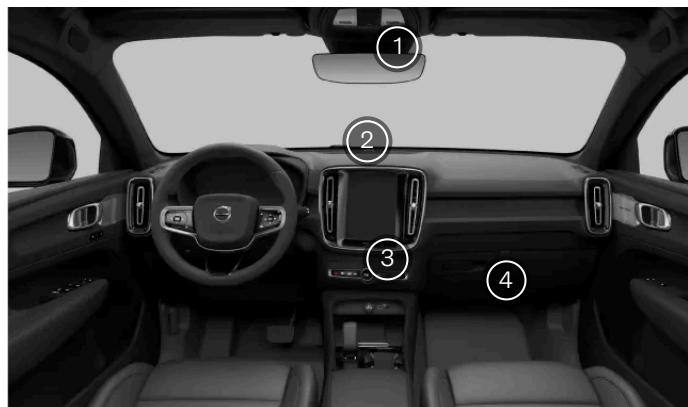
Interior climate sensors
