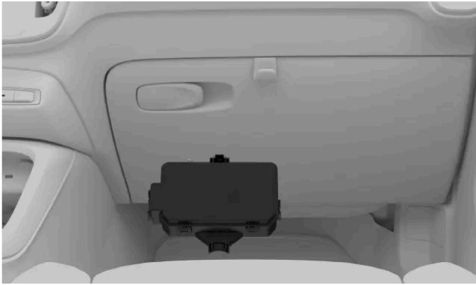
Fuse box location
