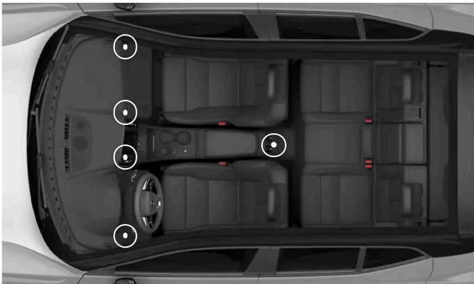
The locations of the adjustable air vents
