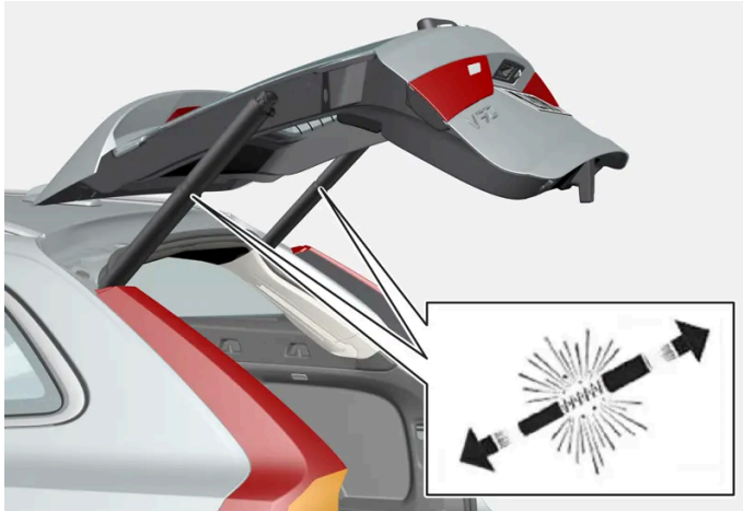
Preloaded springs for the power tailgate.
