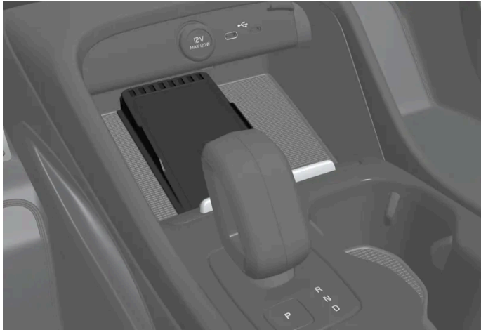
Wireless charger under center display.
