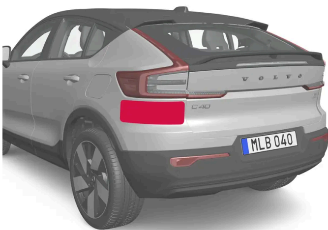
Location of rear radar sensors
