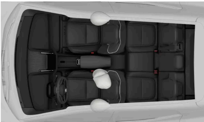
Side-on collision airbags for the front occupants.
