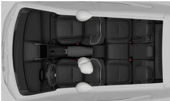
Side-on collision airbags for the front occupants.
