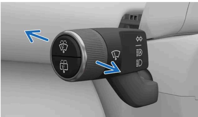
You can move the left-hand stalk forward or backward to switch between the different high beam options. The stalk always springs back to the neutral position.
