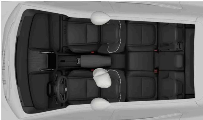
Side-on collision airbags for the front occupants.
