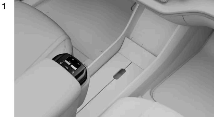
From the front seats, you can control all of the power windows. Press the button with the text REAR to switch between operating the front or rear windows. The button turns amber to indicate that the rear windows are selected. The controls will switch back to the front windows if you press the button again or after a few seconds of inactivity.
