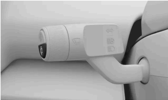
You control the rear windshield wiper by using the lower button on the left-hand steering wheel stalk.
