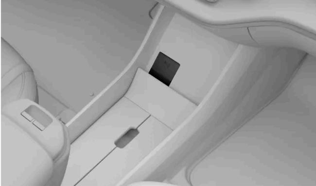
The location of the key card reader used to start the vehicle with a key card or a discharged distance-capable key.
