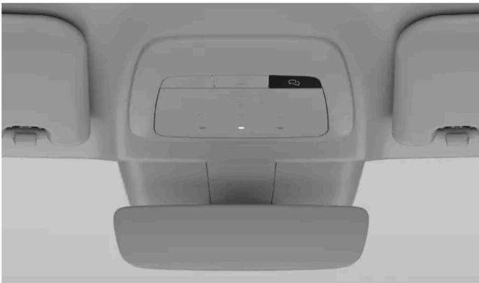
The assist button is located on the roof, to the right of the overhead console.
