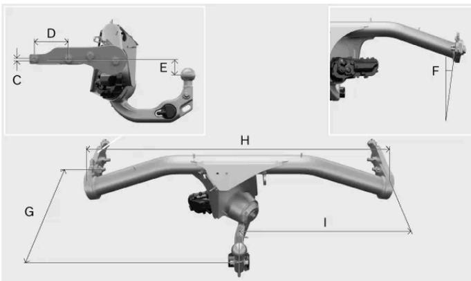
Dimensions, mounting points in millimeters (inches)
