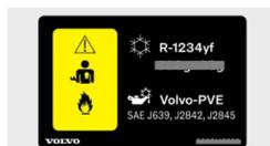
The label with information on climate system fluids is located under the hood, on the right-hand side of the vehicle.
