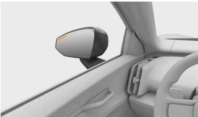
When the vehicle detects traffic that is about to pass close to the vehicle's sides, a light appears in the door mirror along with a notification in the display. If you begin to open the door on the side of the detected traffic, the alert intensifies. An audible alert can occur along with the visual alerts, depending on how urgent the warning is.
