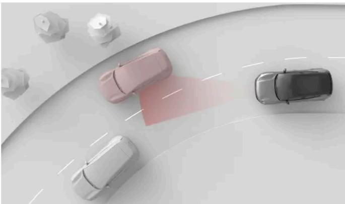
On a curve, the vehicle ahead may slip out of the detection zone. Vehicles in the adjacent lane may also enter the zone, affecting your vehicle's perception of the distance to traffic ahead.
