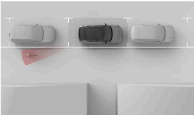
Door opening alerts are designed to warn you of passing traffic so that you don't open a door in its path. These alerts can be provided when the vehicle is stationary or moving very slowly<sup>[1]</sup>.
