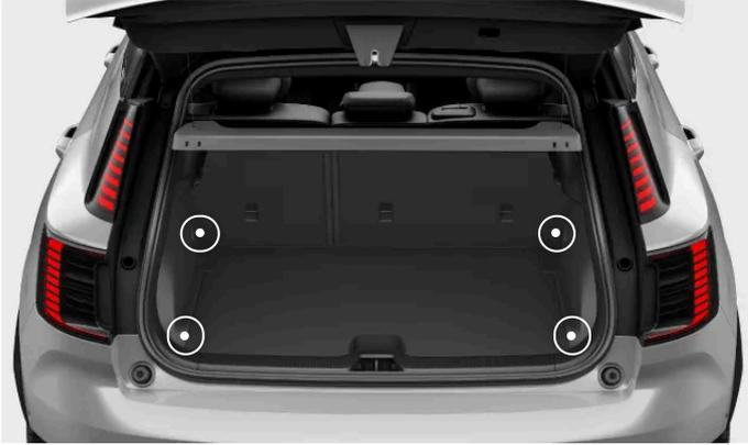
Load-retaining eyelets are located in the four corners of the trunk. You can use the load-retaining eyelets to attach straps and secure cargo in the trunk.
