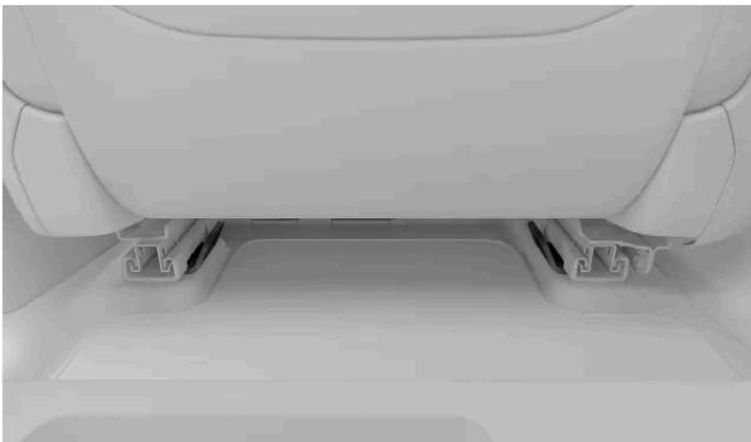
The lower tether attachment points for the rear seats can be found at the back of the floor rails of the seats in front.
