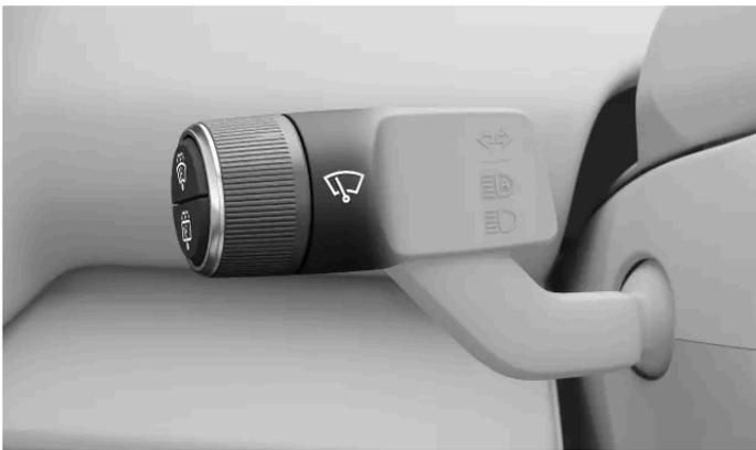
You can control the wipers and washers using the scroll wheel and buttons on the left-hand steering wheel stalk.
