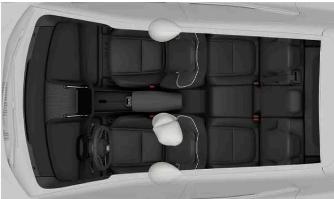
Side-on collision airbags for the front occupants.
