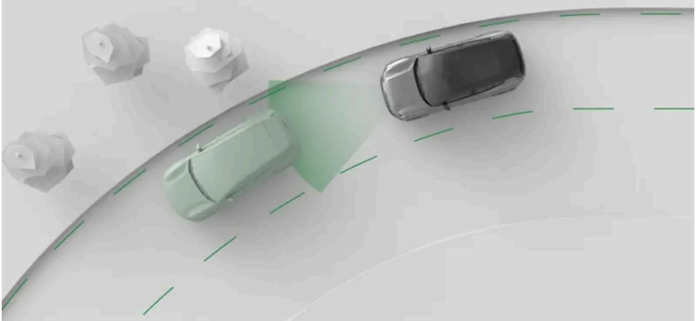
Pilot Assist actively guides your driving in a number of ways. When driving with Pilot Assist, you select the target speed. The vehicle then manages acceleration and braking to meet that target while also adapting to surrounding traffic.
