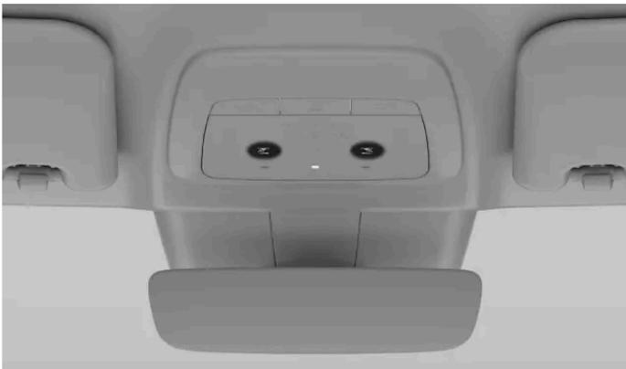
The front seat reading lights in the overhead console
