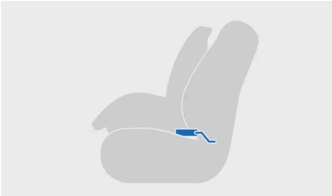
Child restraint installed using ISOFIX<sup>[1]</sup>
