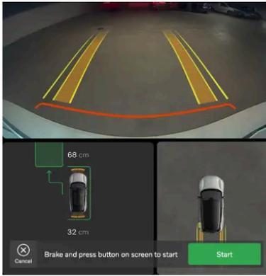
2 To confirm the path and start the maneuver, press the **Start** button in the display.
