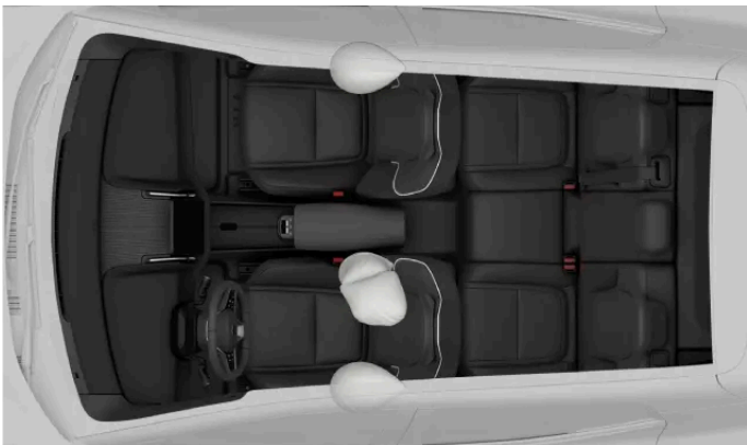
Side-on collision airbags for the front occupants.
