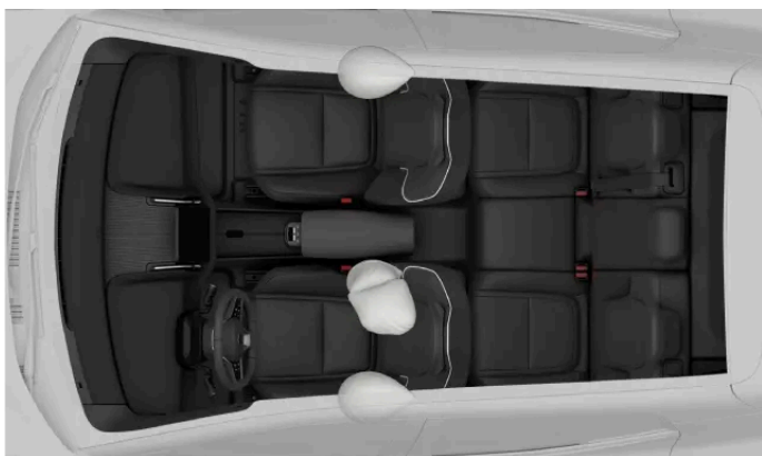
Side-on collision airbags for the front occupants.
