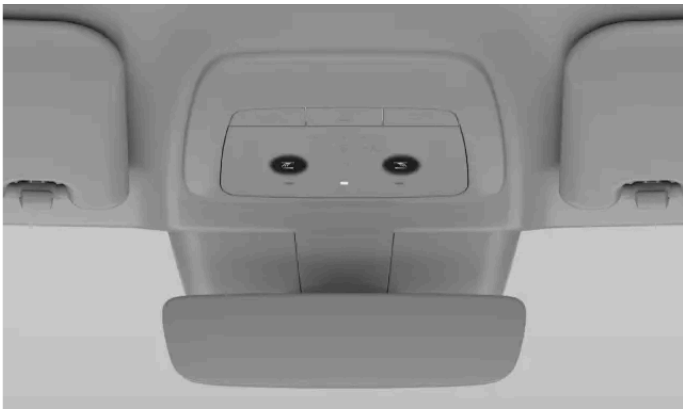
The front seat reading lights in the overhead console
