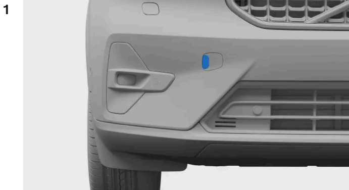
Front towing eye fastening cover
