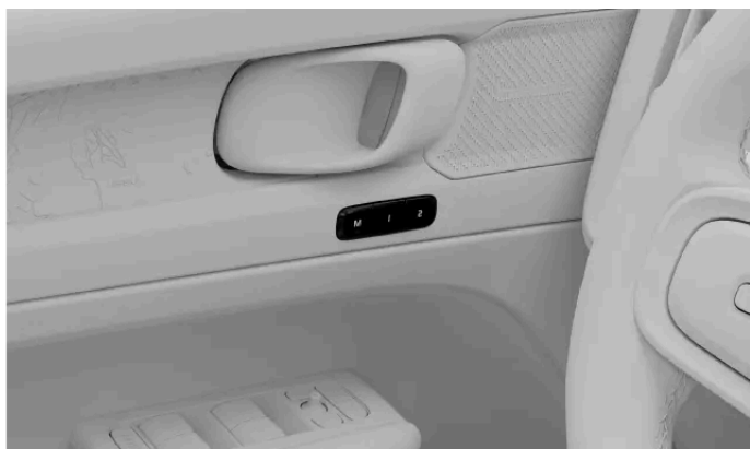
Location of the preset seat adjustment buttons
