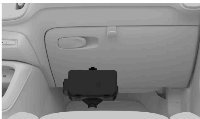
Fuse box location
