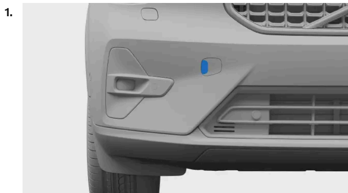
Front towing eye fastening cover
