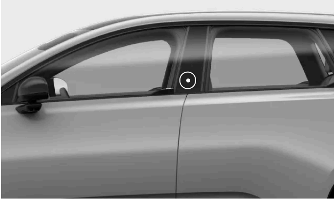
Location of the key reader on the door pillar
