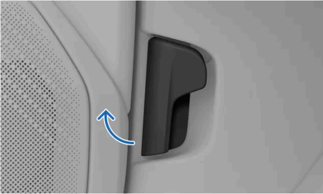
Pulling the interior release lever
