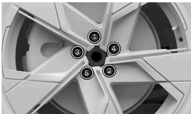
Tighten the wheel fasteners crosswise.
