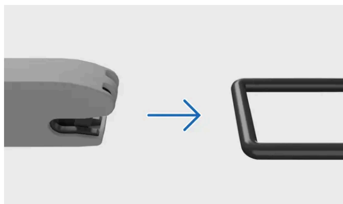
Attaching to ISOFIX [1] attachment point
