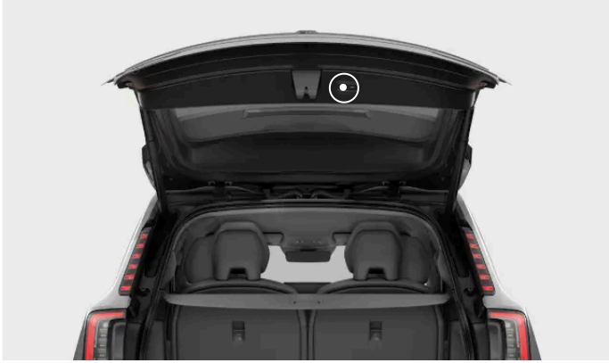
Location of the trunk closing button
