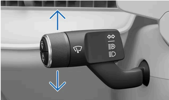
You can control the indicators using the left-hand stalk
