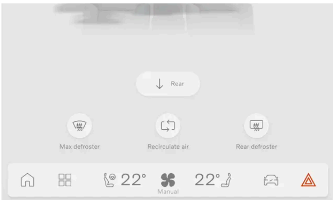
The location of the hazard lights button in the center display
