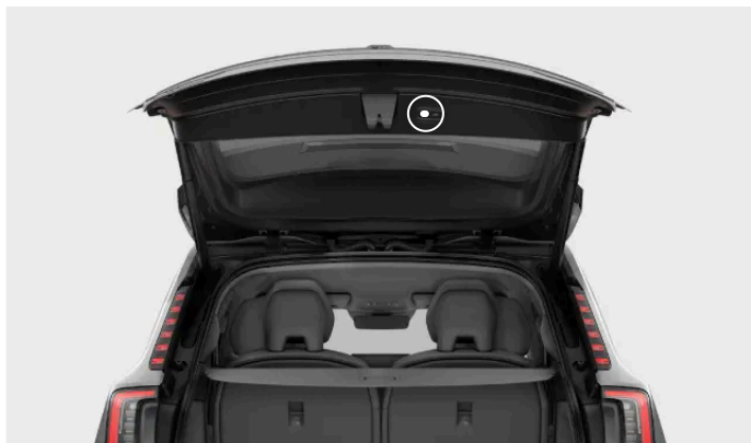
Location of the trunk closing button
