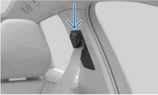
Seat belt top attachment point.
