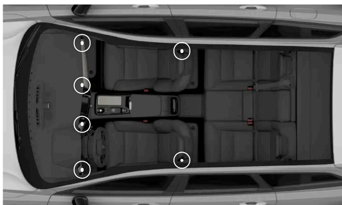
The locations of the adjustable air vents
