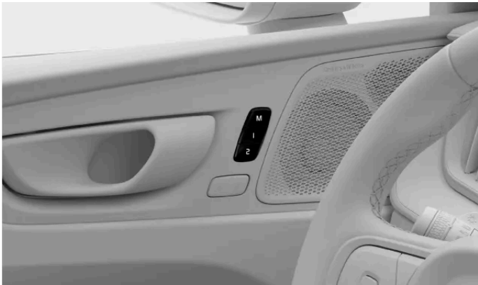
Location of the preset seat adjustment buttons
