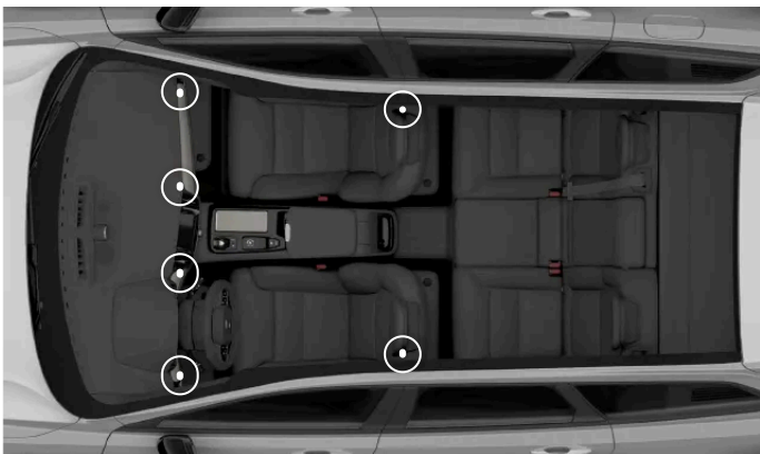
The locations of the adjustable air vents
