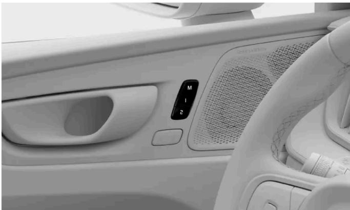
Location of the preset seat adjustment buttons
