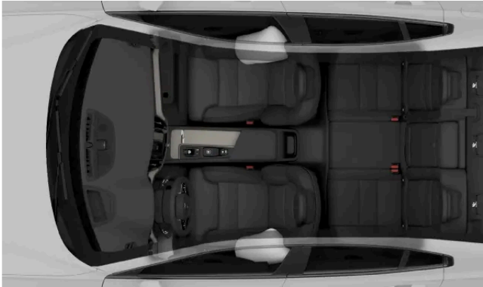
Side-collision airbags for the front occupants.
