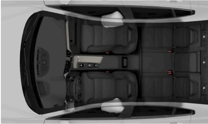
Side-collision airbags for the front occupants.
