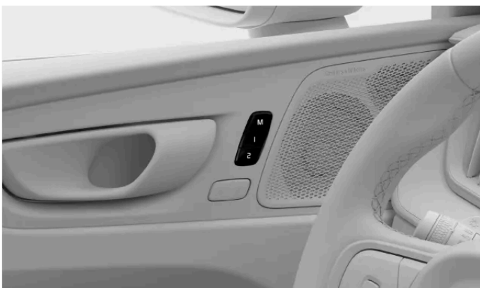
Location of the preset seat adjustment buttons
