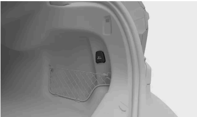
The 12 V electrical outlet on the right side of the trunk
