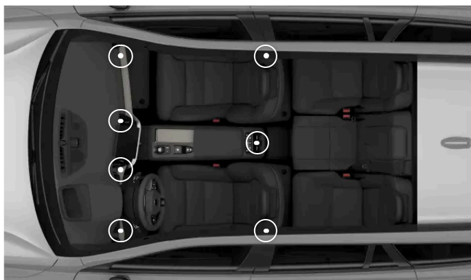
The locations of the adjustable air vents
