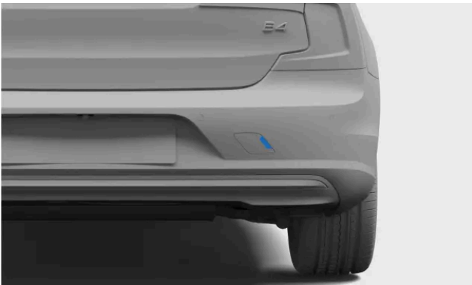
Rear towing eye fastening cover
