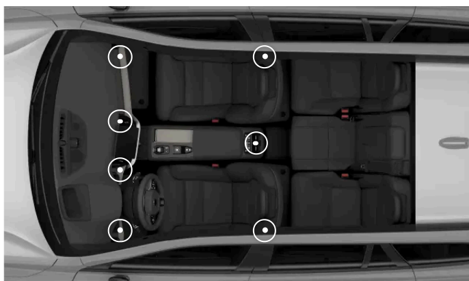
The locations of the adjustable air vents
