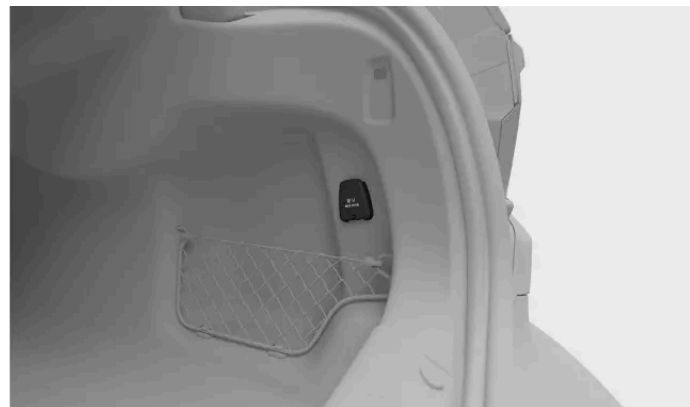
The 12 V electrical outlet on the right side of the trunk
