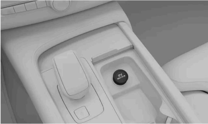
The 12 V electrical outlet in the center console
