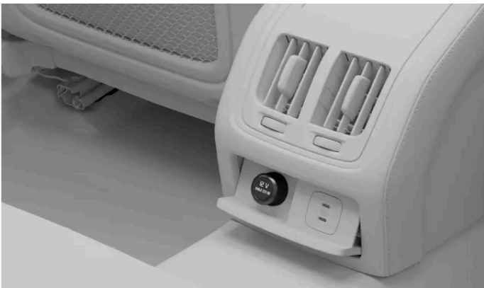
The 12 V electrical outlet in the center console
