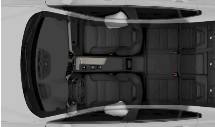
Side-collision airbags for the front occupants.
