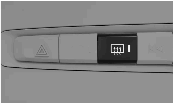
Rear defroster button on the button panel below the center display
