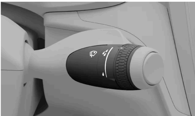
Front wiper controls are on the right-hand steering wheel stalk.
