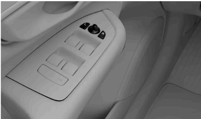
Controls for adjusting the door mirrors
