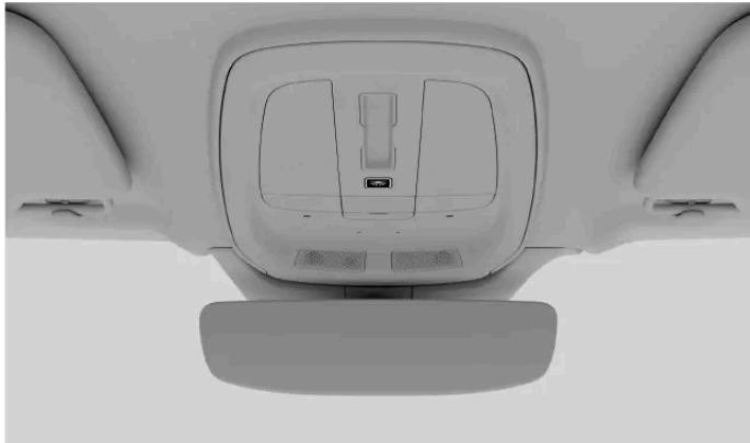
All interior lights on button in the overhead console
