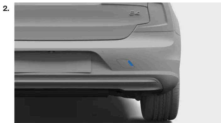
Rear towing eye fastening cover
