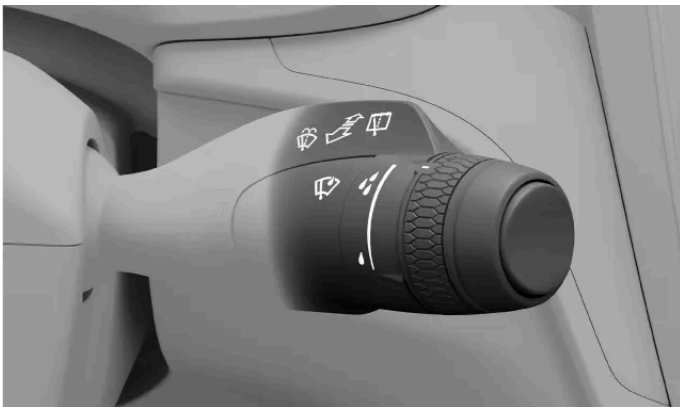
Right-hand steering wheel stalk
