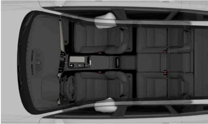
Side-collision airbags for the front occupants.
