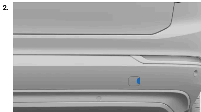
Rear towing eye fastening cover
