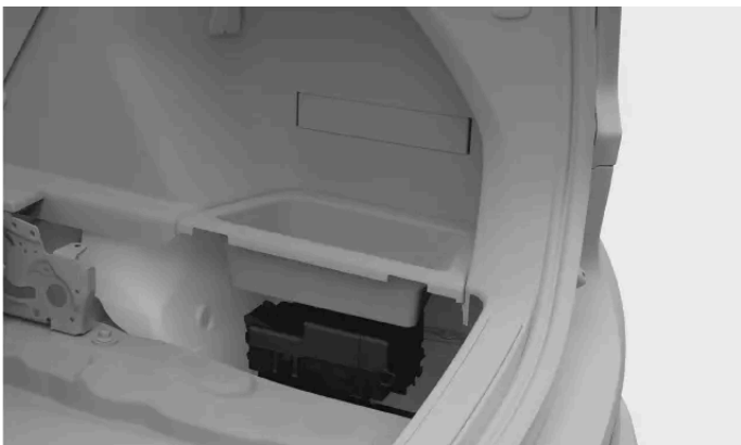
Fuse box location
