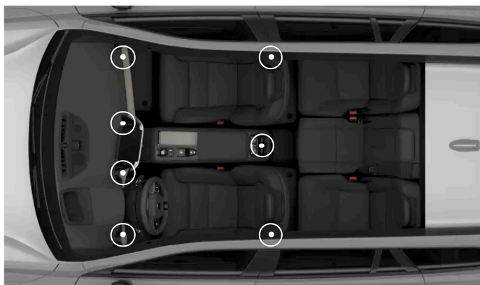
The locations of the adjustable air vents
