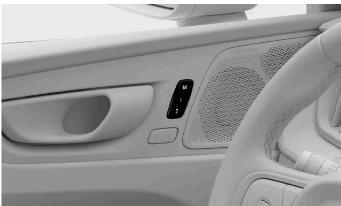
Location of the preset seat adjustment buttons
