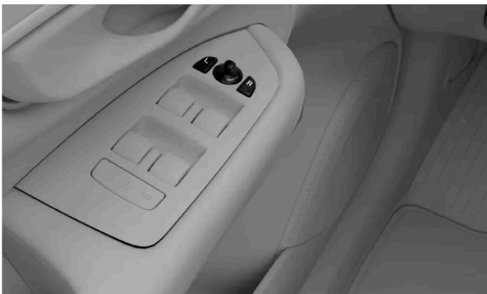
Controls for adjusting the door mirrors
