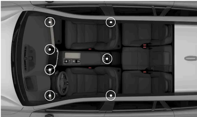
The locations of the adjustable air vents
