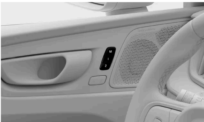
Location of the preset seat adjustment buttons
