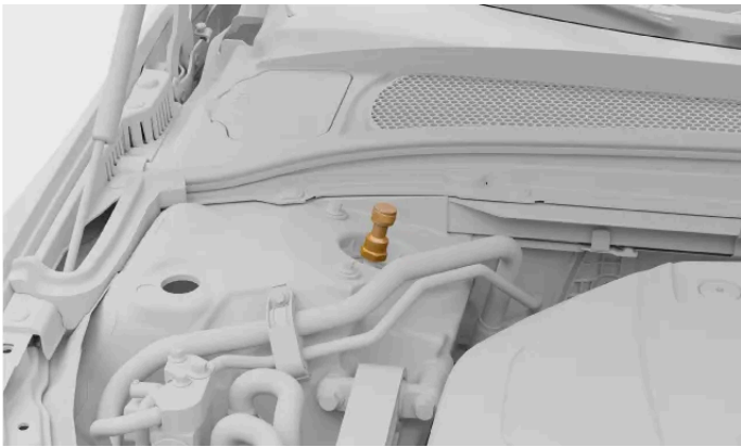
The front wheels' suspension adjustment knobs are located under the hood.
