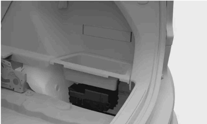
Fuse box location
