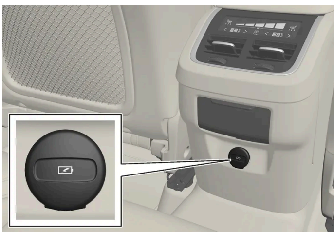
USB ports (type C) on rear of tunnel console for charging devices such as phones and tablets [1] .
