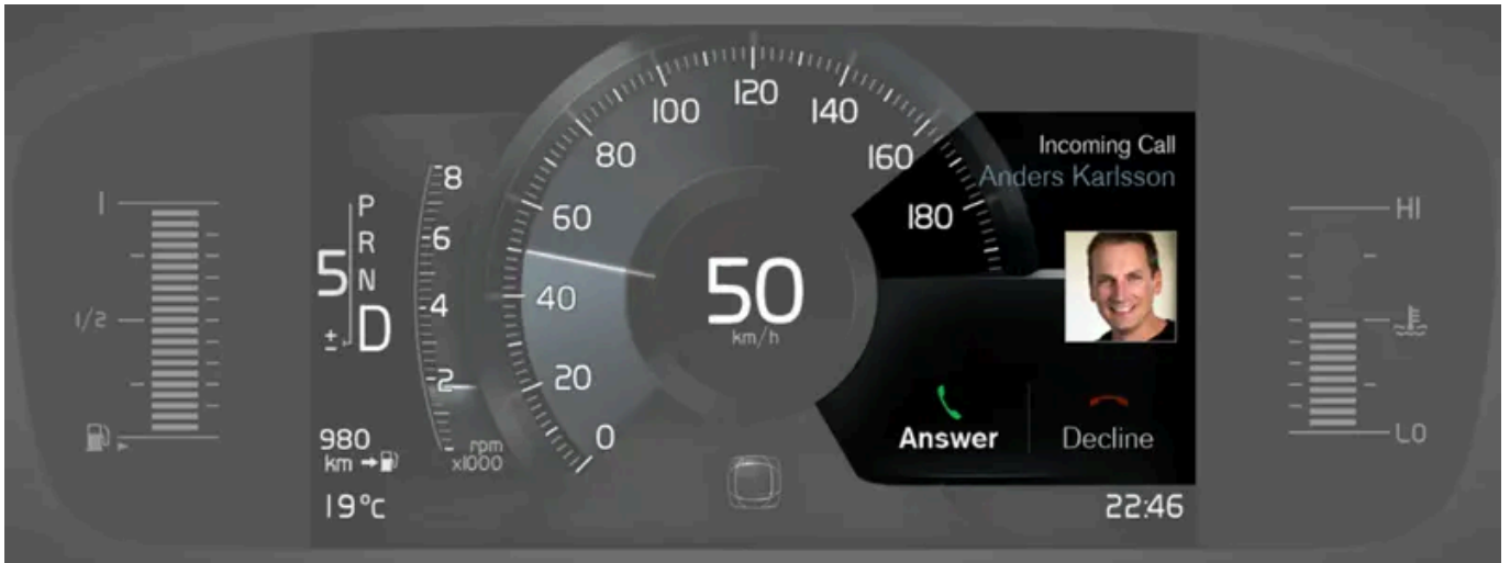
Example of message in an 8-inch instrument panel. The illustration is generic - details may vary according to vehicle model.
