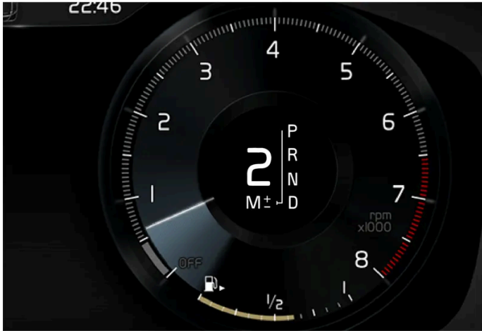
Overview of gear shift pattern in the instrument panel for large gear selector.
