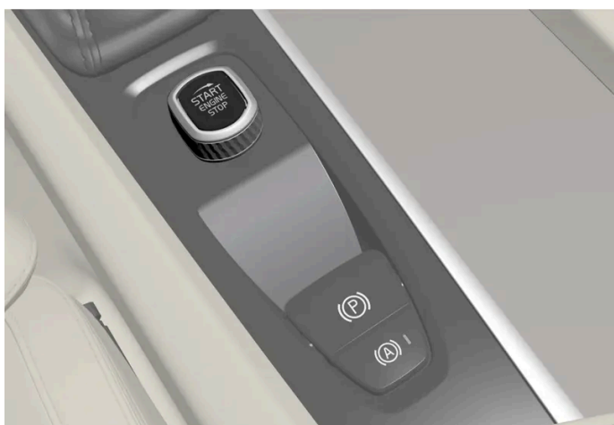
Start knob in the tunnel console.
