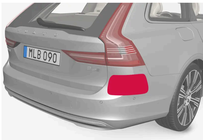
Location of rear radar sensors
