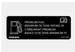
Illustration 2: Decal on the inside of the fuel filler flap on vehicles that require premium fuel [2] .
