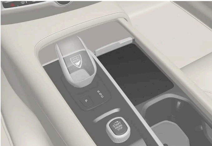
Wireless phone charger in the tunnel console.
