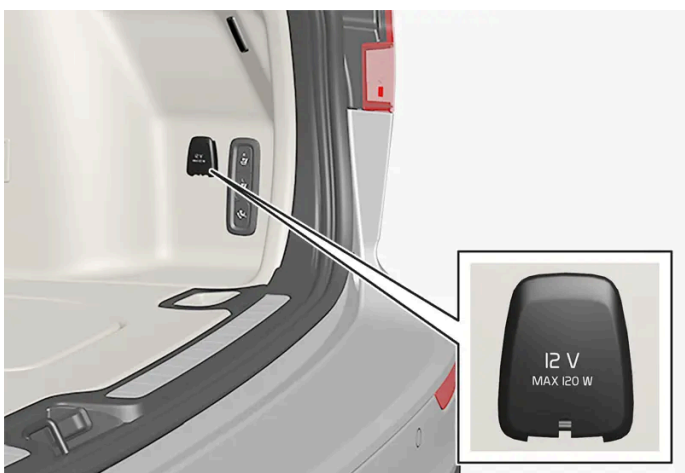
12 V outlet in trunk/cargo compartment*.
