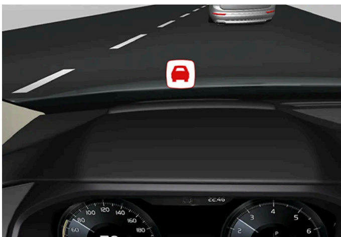
Collision warning symbol on the windshield
