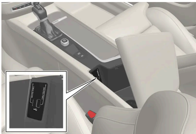
USB ports (type A) in the tunnel console. Route the cable forward to help avoid pinching when the cover is closed.
