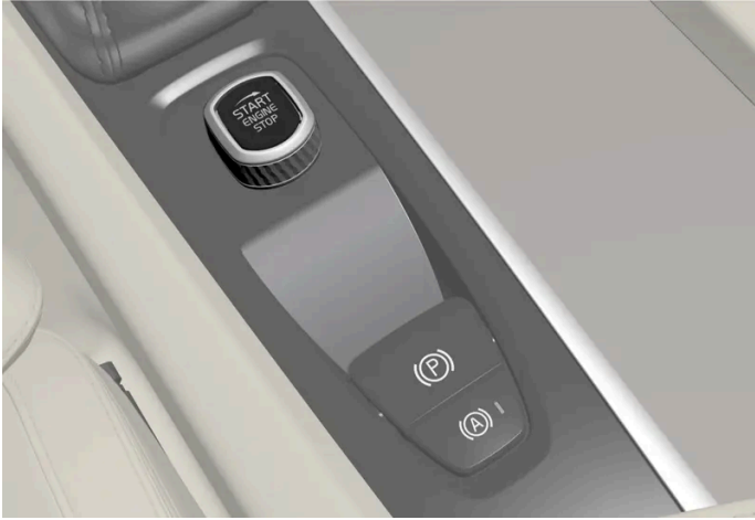
Start knob in the tunnel console.
