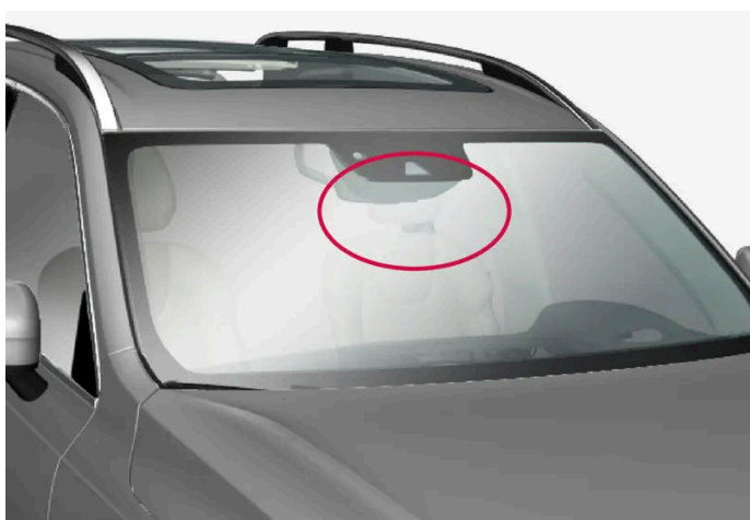
Location of front camera and radar sensor
