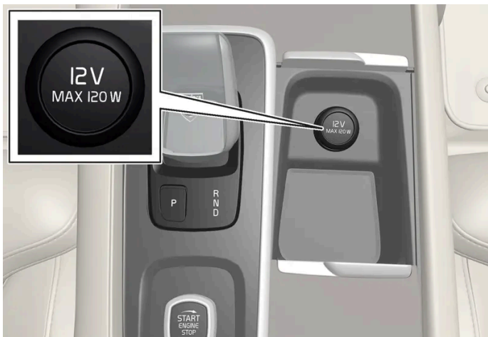
Front electrical outlet in the tunnel console for vehicles without wireless phone charger*.
