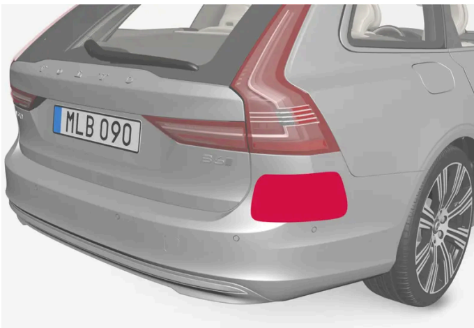
Location of rear radar sensors
