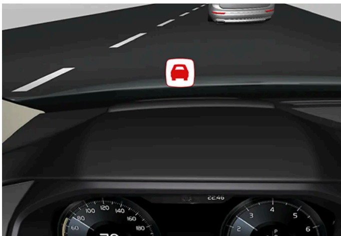
Collision warning symbol on the windshield
