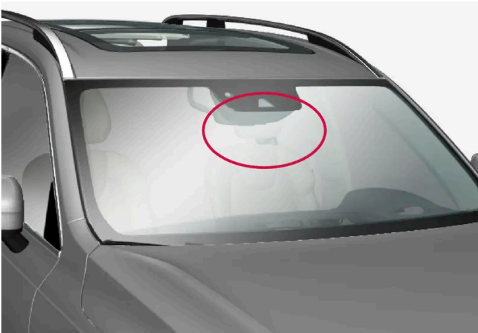
Location of front camera and radar sensor
